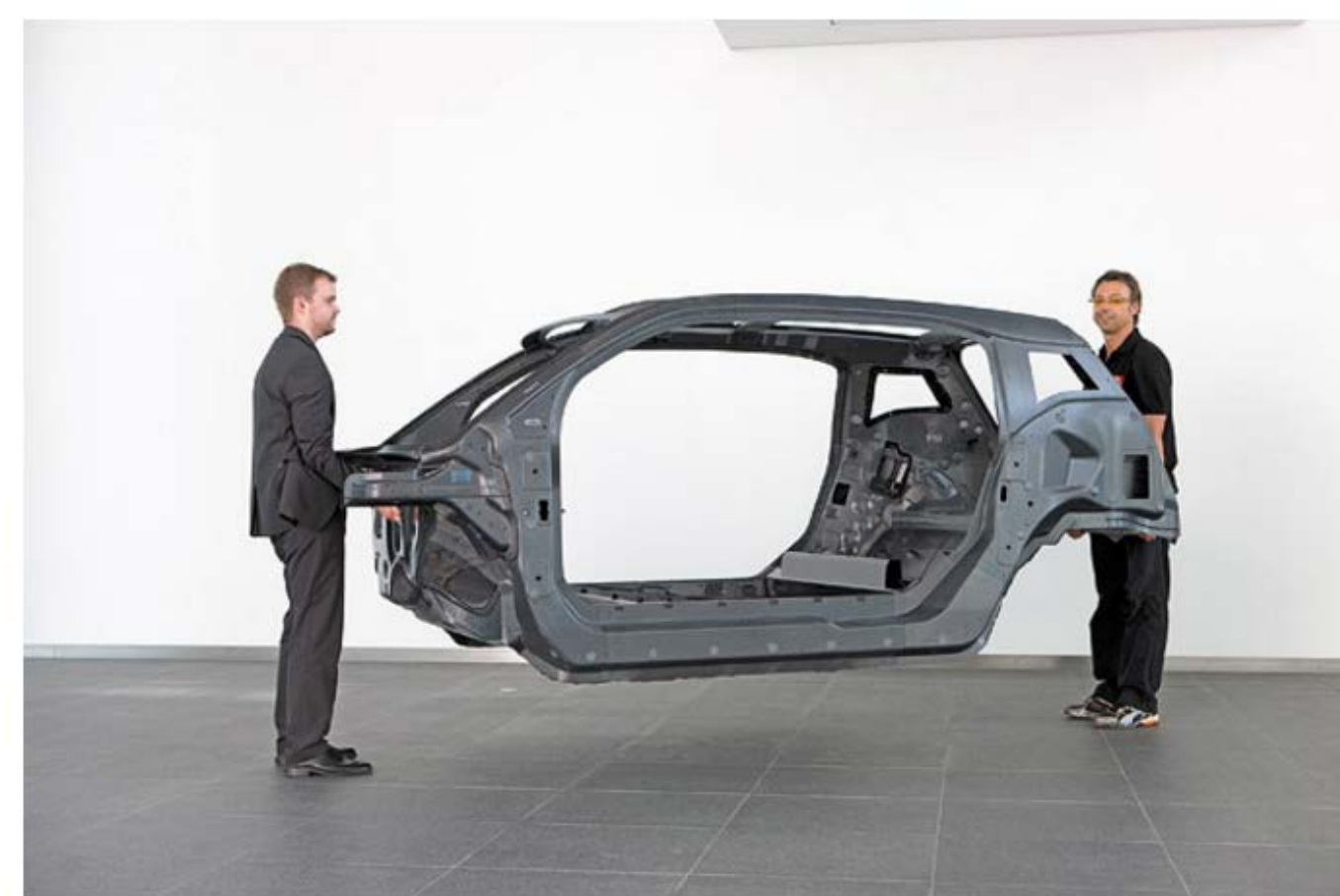
The passenger frame of BMW's i3 is fashioned from lightweight carbon fiber. Courtesy: Auto Bild/Robert Sporn, Germany
